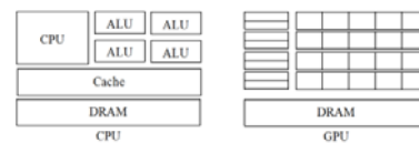
Fig. 1 Difference Between CPU and GPU Architecture [1]
