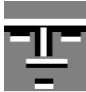
Fig. 4 Applying HAAR Features on Face
